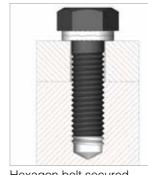
Hexagon bolt secured in a blind hole
