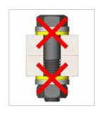
HEICO-LOCK® HLK-Washers are a direct substitute for the commonly used plain chamfered washers according to DIN EN 14399-6. No locking function will be achieved when the HLK-Washers are combined with additional washers or fasteners!
