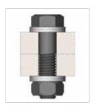
HV sets need to be secured on both sides of a through-hole: One pair of HEICO-LOCK® HLK-Washers under the bolt head and one pair under the nut body.
