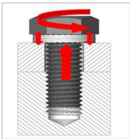
Figure 7: Increase of clamp load during loosening
